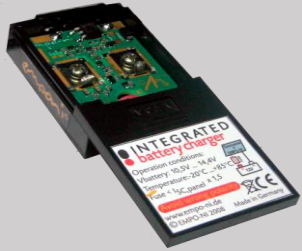
Solar panel integrated battery charger (5Wp-80Wp 12V-48V)
