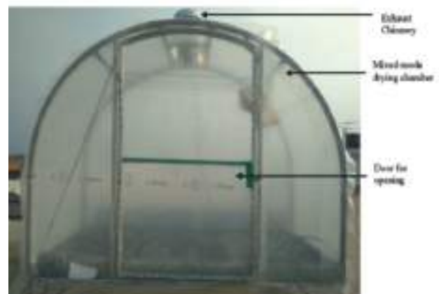
Figure 4.5 Photographs of the developed mixed-mode solar dryer installed for rubber sheet drying with front- and back-side views of drying chamber.
