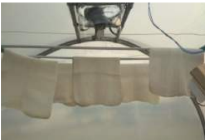
Figure 4.3 Natural rubber sheets hung for drying inside the solar dryer
