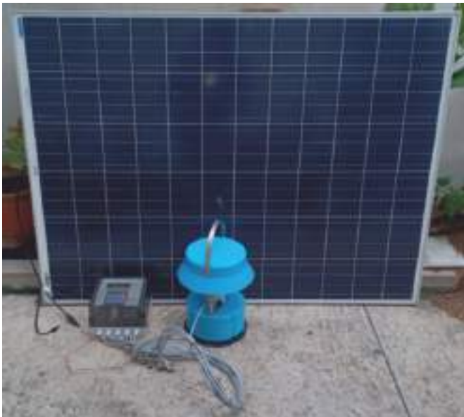
Figure 6.2: Portable solar system for charging digital equipment
